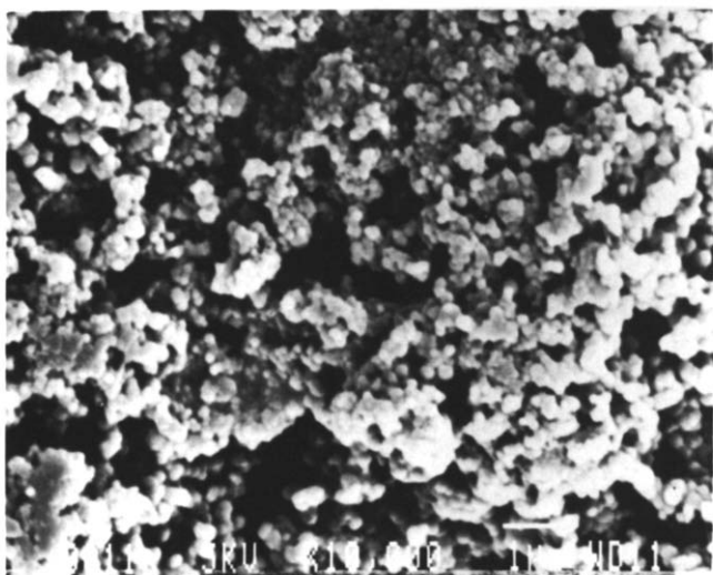
Figure 7 Scanning electron micrograph of the internal fracture surface of the n-propanol extracted 30% polyurea-polyether blend
